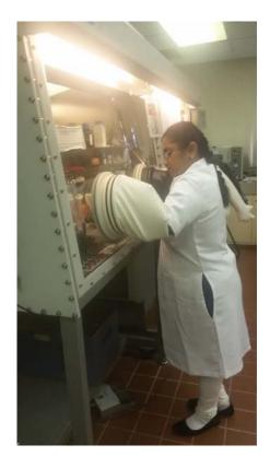
The so-prepared coin cells were taken out of the glove box, cleaned with acetone to remove any electrolyte that could have seeped outside the cell, numbered and the open circuit voltage of the cell to test proper assembling.
